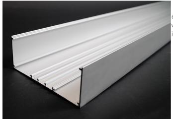
6063-T5 extruded aluminum, satin anodized finish, .080'' (2.03mm) wall thickness. Base has four ribs for snap-in divider. AL5200B-5 is packed eight 5' (1.5m) lengths per carton. Made in U.S.A.
