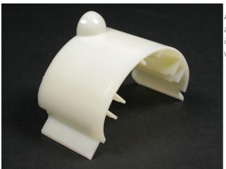
A radiused insert for the ALA3811 and ALA4811 flat elbow to provide a bend radius of 2'' (51mm) for Fiber Optic/Category 5e installations. The insert is ideal for new and retrofit applications whether the cable installation is lay-in or pull-through.
