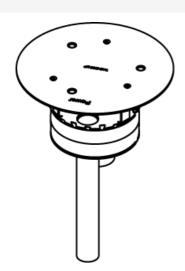
Use with AMD8C Series Covers to complete installation. AMD8 Series Poke-Thru Devices require a 4" (102mm) diameter hole. Not designed to work with bare concrete or terrazzo. Floor covering thickness 1/8" minimum.
