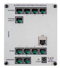
The Audio Distribution Module is used to connect up to four sources to the On-Q Digital Audio System and distribute those sources to four zone outputs. It can be expanded to accommodate up to sixteen sources and sixteen zo
