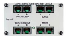
The Digital Audio Expansion Module expands the capabilities of Legrand's Digital Audio Distribution Module (<u>AU7000</u>), offering four additional zones (rooms) within a Digital Audio S
