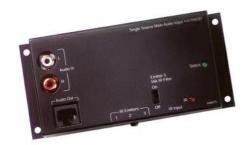
The Single Source Input typically resides at the entertainment center and is connected to the enclosure mounted Audio Distribution Module using a single Category 5 cable run. This Single Source Input requires line level output from the audio source bei
