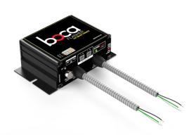
The BF-SDS10V-AST takes a 0-10V dimming signal and a fixed line voltage input and converts it to a phase-adaptive dimmed output for up to 1300W for a 277V load and 750W for a 120V load. The dimming type used (forward phase or reverse phase) is automatically selected by the BF-SDS10V-AST for optimal dimming performance. The BF-SDS10V-AST has a built-in slotted mounting bracket for surface mounting and is rated for install in plenum spaces
