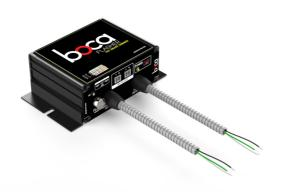
The BF-SDS10V-AST takes a 0-10V dimming signal and a fixed line voltage input and converts it to a phase-adaptive dimmed output for up to 1300W for a 277V load and 750W for a 120V load. The dimming type used (forward phase or reverse phase) is automatically selected by the BF-SDS10V-AST for optimal dimming performance. The BF-SDS10V-AST has a built-in slotted mounting bracket for surface mounting and is rated for install in plenum spaces
