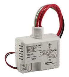
The BZ-200 power pack switches connected loads On and Off in response to Wattstopper low voltage occupancy sensors. It also provides up to 225mA at 24VDC to power the sensors. This device is constructed with environmentally friendly materials and is RoHS-compliant.
