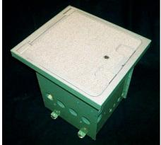
For use with the CCFB Series™ Convention Center Type LS boxes, the CCFBC-NS-H-C4 is a cover assembly with a solid top cover with non skid texture. The cast aluminum cover assembly is load tested to support over 32,000 pounds with a safety factor of 2(64,000 lbs.). The cover is hinged to open a full 180 degrees and meet the UL scrubwater requirements.
