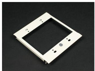
For installation of two-gang devices or two vertically mounted single-gang devices on undivided raceway. Use with industry standard double-gang faceplates for electrical and communication devices. Can also be used with 4000B Series. Certified to Canadian Safety Standards for sale in Canada. When ordering these products, change the "V" color prefix to "CV" or the "G" color prefix to "CG" to denote the Canadian versions.
