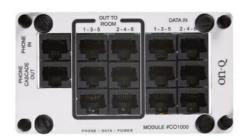
Allows the distribution of phone and data to up to six rooms with the convenience of a single pull of Cat 5e cable. Supports up to two phone lines and one 100BASE-T data connection per pull. The WP1000 phone/data strap is required on outlets to complete the solution.
