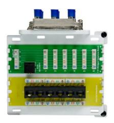
The Trio Combo Module with Cat6 Data is designed to distribute video (Coax), voice (Telephone), and data (Ethernet) services from a single, compact structured wiring module. This module ensures high-speed and reliable performance throughout your home. It includes an MDU Mounting Bracket (AC1042), an 8-way passive digital HDTV cable splitter (VM0208), a 6-way Phone Module (TM0106), and a 6-way Cat 6 Data Board (AC0606) for comprehensive connectivity.
