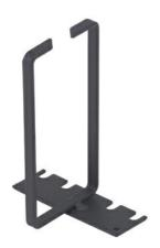
CR-93S-1B and CR-93S-3B rings fit within the width of a rack; they are designed for smaller, single-rack installations or where the width of the rack cannot be exceeded. Larger capacity CR-93S-2B and CR-93S-4B rings mount between adjacent racks and equal the combined width of the rack channels; they are designed for multiple rack installations
