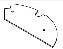
Wiremold CRFB Series Blank Device Plate #2 Part No. CRFB-B-2
