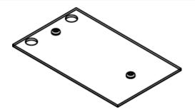
The CRFB4 has four compartments that accept different device plates. This Blank Device Plate is for Plate location 4, used to close off unused gang. NOTE: Standard size for device plates for Plate Location 4 is 5 7/32" (132mm) x 2 3/4" (62mm).
