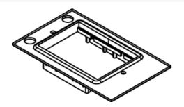
The CRFB4 has four compartments that accept different device plates. This 6A Communication Plate is for Plate location 4, includes: (1) 6A Wiremold Open System Adapter, (1) Ortronics Series II Adapter, (1) Ortronics TracJack Adapter. Modular jacks sold separately. NOTE: Standard size for device plates for Plate Location 4 is 5 7/32" (132mm) x 2 3/4" (62mm).
