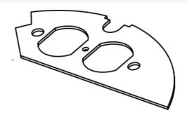
The CRFB4 has four compartments that accept different device plates. This Duplex Device Plate is for Plate location 2, accepts standard 15A and 20A duplex receptacles. NOTE: Standard size for device plates for Plate Location 2 is 5 7/32" (132mm) x 2 3/4" [62mm].
