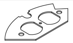
The CRFB4 has four compartments that accept different device plates. This Duplex Device Plate is for Plate location 3, accepts standard 15A and 20A duplex receptacles. NOTE: Standard size for device plates for Plate location 3 is 6 11/32" (161mm) x 2 3/4" (62mm).
