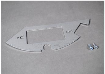
The CRFB4 has four compartments that accept different device plates. This GFCI/Decorator Device Plate is for Plate location 1, accepts standard GFCI or Decorator style receptacles. NOTE: Standard size for device plates for Plate Location 1 is 6 11/32" [161mm] x 2 3/4" [62mm].
