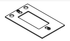
The CRFB4 has four compartments that accept different device plates. This GFCI/Decorator Device Plate is for Plate location 4, accepts standard GFCI or Decorator style receptacles. NOTE: Standard size for device plates for Plate Location 4 is 5 7/32" (132mm) x 2 3/4" (62mm).
