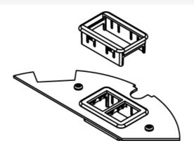
The CRFB4 has four compartments that accept different device plates. This Communication Device Plate is for Plate location 1, accepts two (2) ports of communication devices. Includes one (1) Ortronics Series II and one (1) Tracjack adapter. NOTE: Standard size for device plates for Plate Location 1 is 6 11/32" [161mm] x 2 3/4" (62mm).
