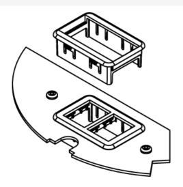
The CRFB4 has four compartments that accept different device plates. This Communication Device Plate is for Plate location 2, accepts two (2) ports of communication devices. Includes one (1) Ortronics Series II and one (1) Tracjack adapter. NOTE: Standard size for device plates for Plate Location 2 is 5 7/32" (132mm) x 2 3/4" (62mm).
