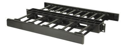
Legrand® standard horizontal cable managers are available in 1RU and 2RU sizes. Fingers begin 3/4" from the face of rack to provide bend limitation for cables, protecting cables, equipment and network performance. Included hinged cover mounts with six heavy duty clips allow them to be opened one handed without becoming "unhinged". Manufactured from UL94V-0 rated plastic.
