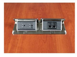
Unit includes one (1) 15A black tamper-resistant duplex receptacle. Second opening will accept adapter for one (1) Wiremold CM Series Open System 2A module, one (1) Ortronics Series II or one (1) TracJack adapter to accommodate a wide range of communication outlets. Adapters are included in hardware bag. Unit comes with a 6' (1.83m) cord. Comes with a brushed stainless steel finish.
