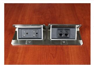
Unit includes one (1) 20A black tamper-resistant duplex receptacle. Second opening will accept adapter for one (1) Wiremold CM Series Open System 2A module, one (1) Ortronics Series II or one (1) TracJack adapter to accommodate a wide range of communication outlets. Adapters are included in hardware bag. Unit comes with a 6' (1.83m) cord. Comes with a brushed stainless steel finish.
