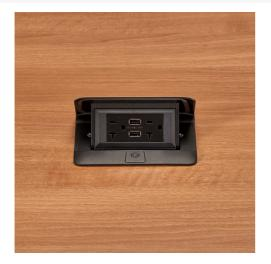
Unit includes one (1) 20A black tamper-resistant duplex receptacle with two (2) USB ports that provide 3.1A. Unit comes with a 6' (1.83m) cord. Comes with a black powder coat finish.
