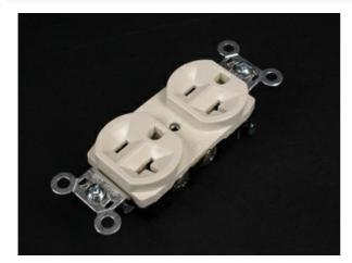
Specification grade rated 20A 125V NEMA 5-20R receptacle. Receptacle has nylon face and thermoplastic base. One-piece brass triple-wipe line contacts and double-wipe ground contacts. Locked in wrap-around steel yoke. Break off tab for two circuit wiring. 2.7" W x 4.5" H (69mm x 114mm). Verified under Fed. Spec. #WC596F.
