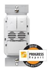
The DW-311 dual technology dimming wall switch sensor can turn lights OFF and ON based on occupancy and allow the user to increase or decrease the lighting level. It combines the benefits of passive infrared (PIR) and ultrasonic occupancy detection technologies and works with 0-10 VDC dimming drivers and ballasts to control lighting loads including LEDs.
