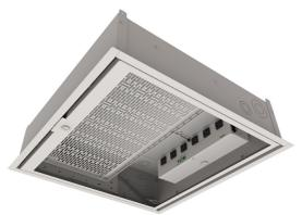
Fully finished enclosure designed to manage and store A/V equipment in an air handling plenum space above a false ceiling. Equipped with dry contact controlled receptacles that can be switched off when not in use and has a built-in fan to keep the temperature of the equipment cool.
