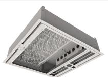
Fully finished enclosure designed to manage and store A/V equipment in an air handling plenum space above a NO ceiling. Equipped with dry contact controlled receptacles that can be switched off when not in use and has a built-in fan to keep the temperature of the equipment cool. Built-in projector mount that utilizes a 1 1/2" standard NFS fitting and is rated to support a load up to 50 lbs.
