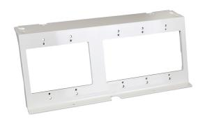
Equipped with one 2-gang standard size device opening and one 3-gang standard size device opening. Accepts a standard 2-gang  $(4.9/16'' \times 4.1/2'' (116mm \times 114mm))$  and a 3-gang  $(6.3/8'' \times 4.1/2'' (162mm \times 114mm))$  device plate.
