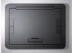
Die cast aluminum cover assembly designed to be used on top of floor covering. Available in the following powder coated finishes: black (BK), gray (GY), brass (BS), nickel (NK) and bronze (BZ). For use on Evolution Series 6-, 8- and 10-gang floor boxes (EFB6, EFB8 and EFB10).
