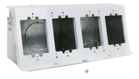
Bank of four (4) compartments that accept power, communications and audio/video devices. Accepts standard size (2 3/4'' x 4 1/2'') (70mm x 114mm) device plates. Includes one device bracket, one back plate, two (2) knockout plates, two (2) end caps and one divider. NOTE: Module will fit on either side of the floor box.
