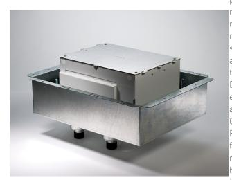
"The Evolution™ Series Eight Gang Fire Classified Floor Box has been designed to be installed in above grade concrete floors while maintaining the fire classification of the floor. This box is classified to be used in 2-hour fire rated floors. Designed to accept standard size wall plates. Box comes complete with all components needed for initial installation. Included components are:
