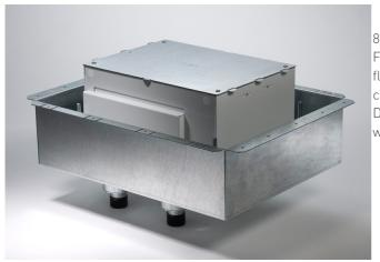
8-Gang Fire Classified Floor Box Pre-assembled installation ready Floor Box has been designed to be installed in above grade concrete floors while maintaining the fire classification of the floor. This box is classified to be used in 1-, 1 1/2-, 2-, or 3-hour fire rated floors. Designed to accept standard size wall plates. Box comes complete with all components needed for initial installation.
