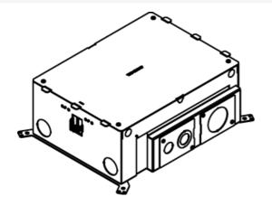
The Evolution™ Series Eight Gang Floor Box has been designed to be installed in concrete, raised, and wood floor applications. The box has a fully finished interior to assist plugging and unplugging of devices. Designed to work with standard size wall plates. It comes complete with all components needed for initial installation. The floor box is compatible with Walkerflex Modular Wiring System. Custom options are available upon request.
