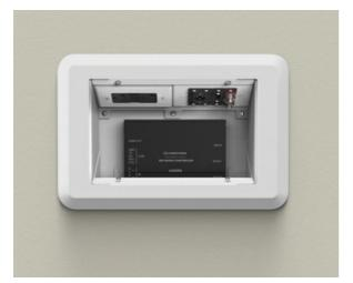
Designed to fit and be concealed behind 42" or larger flat screen displays. Can be installed in both new work and old work applications. Has 2 NEMA size openings for power, communication, or A/V devices. Box is also equipped with a storage module that will accept active A/V equipment up to 6 7/8" x 9 1/8" (175mm x 232mm) (dimensions include wire and cables) in size.
