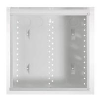
The EN1485 series enclosures include five knockouts on the top of the enclosure. They are also vertically stackable to allow cable passthrough between any two ENxx85 enclosures. For Fiber to the Home (FTTH) applications, it will fit ONTs of 3.6"" depth
