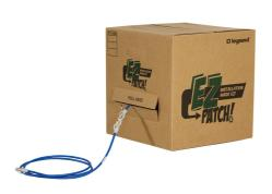
EZ Patch 40 pack, Clarity 6 modular patch cord, blue, 9', Category 6, four-pair UTP stranded 24 AWG PVC/CM, center tuned with Clarity 6 connecting hardware for optimum Category 6 installed performance
