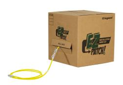
EZ Patch 40 pack, Clarity 6 modular patch cord, yellow, 10', Category 6, four-pair UTP stranded 24 AWG PVC/CM, center tuned with Clarity 6 connecting hardware for optimum Category 6 installed performance
