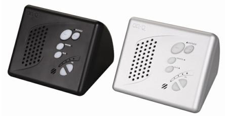
Housed in durable plastic casing, the desk unit brings on-wall unit functionality within arm s reach. It plugs into any RJ45 outlet home run to the enclosure to easily add another room to an intercom system.
