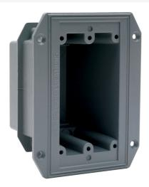
Flanged Box for Horizontal or Vertical Installation, 18.5 Cubic Inch, Minimum Opening Size 2.5\'\' x 4.1\'\' Depth 3.0\'\', Gray
