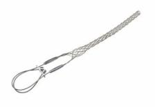
FC062LB: Standard Duty, Closed Mesh, Locking Bale (Universal Eye), Cable Diameter 0.62 - 0.74 inches, Bale Length 18-in, Mesh Length 11-in, Break Strength 1150 lbs.
