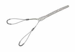
FC062UU: Standard Duty, Closed Mesh, Double -Eye Grip, Cable Diameter 0.62 - 0.74 inches, Bale Length 4-in, Mesh Length 11-in, Break Strength 1150 lbs.
