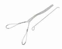
FC075UU: Standard Duty, Closed Mesh, Double -Eye Grip, Cable Diameter 0.75 - 0.99 inches, Bale Length 4-in, Mesh Length 14-in, Break Strength 1320 lbs.
