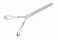
FC100UU: Standard Duty, Closed Mesh, Double -Eye Grip, Cable Diameter 1.00 - 1.24 inches, Bale Length 5-in, Mesh Length 15-in, Break Strength 1920 lbs.
