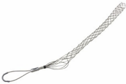
FC175OF: Standard Duty, Closed Mesh, Offset Eye Grips, Cable Diameter 1.75 - 1.99 inches, Bale Length 6-in, Mesh Length 20-in, Break Strength 2640 lbs.
