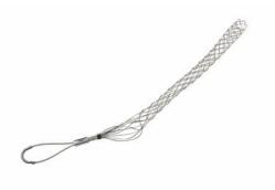
FC1750F: Standard Duty, Closed Mesh, Offset Eye Grips, Cable Diameter 1.75 - 1.99 inches, Bale Length 6-in, Mesh Length 20-in, Break Strength 2640 lbs.
