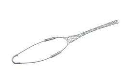
FC175U: Standard Duty, Closed Mesh, Single-Eye Grip, Cable Diameter 1.75 - 1.99 inches, Bale Length 14-in, Mesh Length 20-in, Break Strength 2640 lbs.
