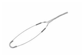
FC30: Bus Drop, Closed Mesh, Single Eye, Cable Diameter 0.30 - 0.43 inches , Bale Length 9-in, Mesh Length 4.5-in, Break Strength 1100 lbs.
