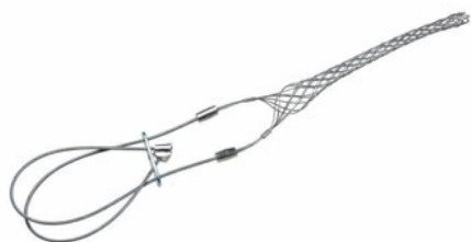
FC40LB: Bus Drop, Closed Mesh, Locking Bale, Cable Diameter 0.41 - 0.56 inches, Bale Length 12-in, Mesh Length 5-in, Break Strength 1100 lbs.
